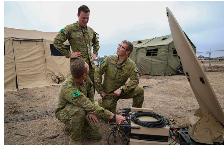
U.S. Soldiers assigned to 86th Expeditionary Signal Battalion, train Australian Forces from 1 st Combat Signal Regiment on setting up the Terrestrial Transmission Line of Sight Radio System as a part of Project Convergence 2022 (PC22) at Camp Pendleton, California, October 7, 2022.
